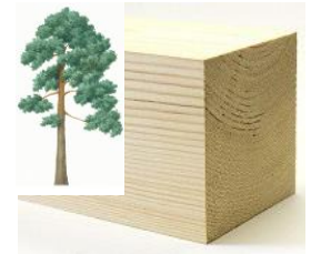
Scots pine - A straight-grained softwood but knotty. Light in colour. Fairly strong but easy to work with. Cheap and readily available.
